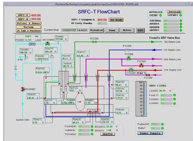
Figure 2: SRF Cavity Test station Flowchart
