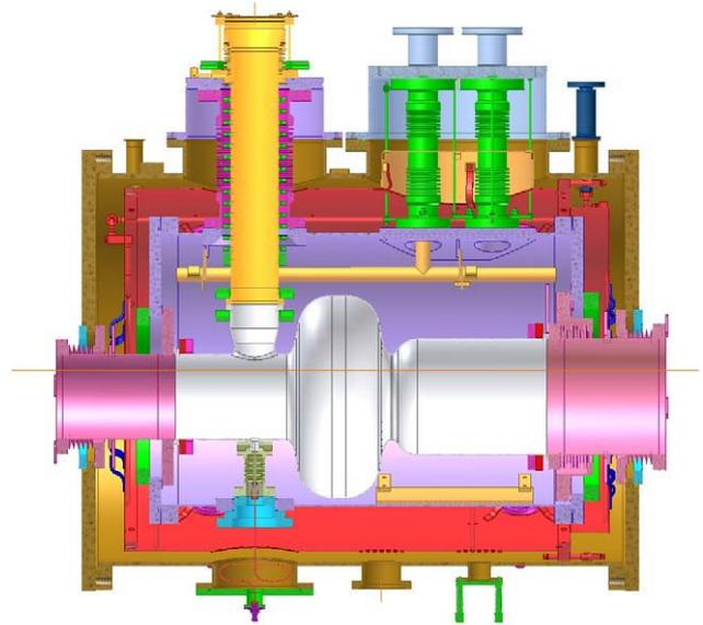
Figure 1: The section figure of SRF cavity and its cryomodule
