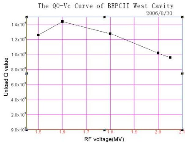
Figure 5: The Q<sub>0</sub>-V<sub>c</sub> Curve of BEPCII West Cavity
