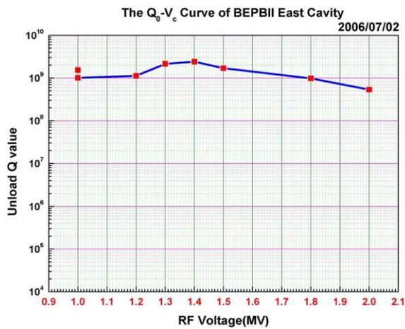
Figure 4: The Q<sub>0</sub>-V<sub>c</sub> Curve of BEPCII East Cavity
