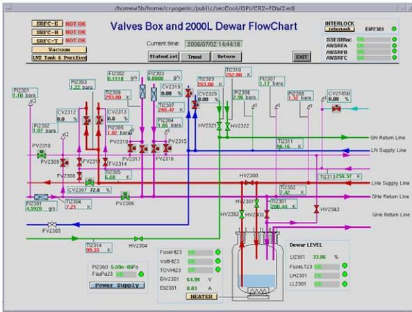
Figure 3: Valves Box and 2000L Dewar FlowChart
