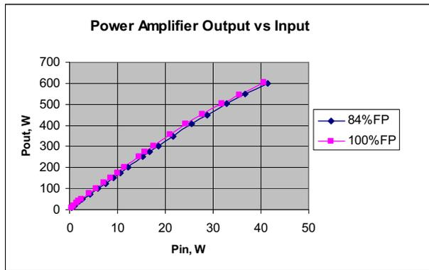
Figure 4: Output power of final power amplifier with different filament powers
