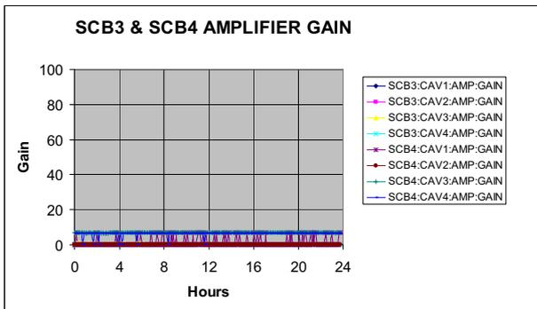
Figure 6: Gain of amplifiers in SCB3 and SCB4 obtained from EPICS archive
