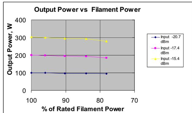
Figure 3: Output power of amplifier with varying filament power
