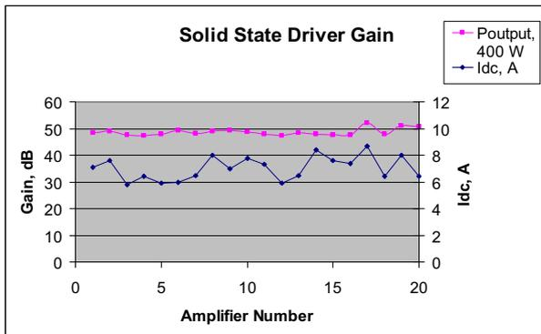
Figure 2: Amplifier gain and dc current for solid state driver amplifiers for 400 Watts output from the power amplifier
