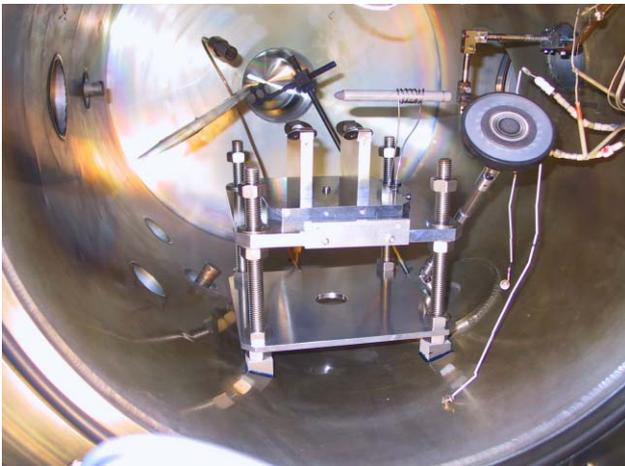
Fig.7 Tapered  $MgB_2+Mg$  target set inside PLD vacuum chamber
