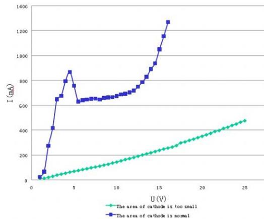
Fig 8. I-V curves with different cathode areas, the blue curve is normal. Much small area of cathode let the green curve like a line
