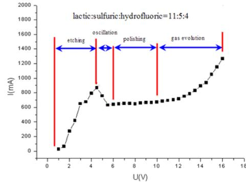
Anode current measured as a function of applied for polishing Nb sample
