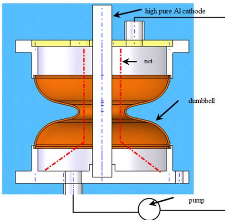
Fig3 Schematic device of BEP for dumbbell
