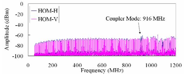
Figure 7: Beam-induced RF spectrum in the beam pipe.
