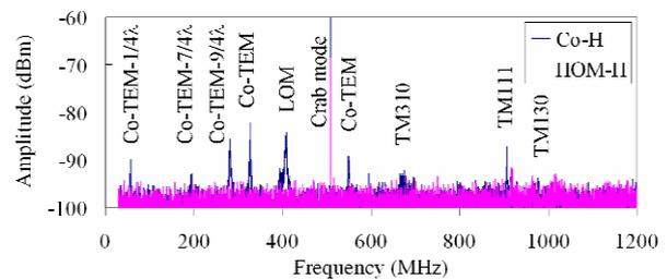
Figure 3: Beam-induced RF spectrum in the single-bunch operation and identified parasitic modes.
