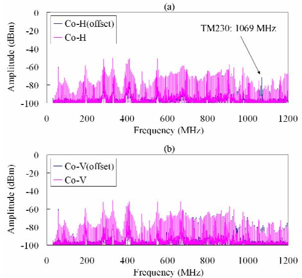
Figure 6: Beam-induced RF spectrum in the horizontal beam offset (a) and in the vertical beam offset (b).
