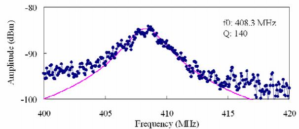
Figure 4: Q and  $f_0$  of the LOM measured in the spectrum.
