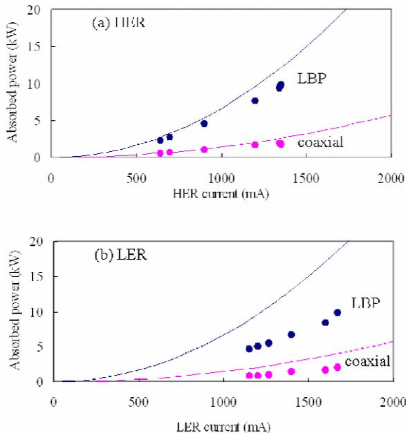
Figure 8: Absorbed HOM power in HER (a) and LER (b). Lines in the figure are calculated power from the loss factor.
