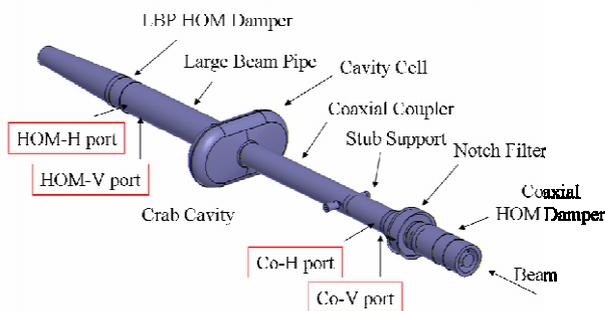
Figure 2: Layout of pick-up ports.
