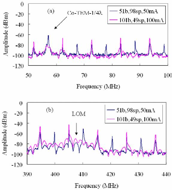
Figure 5: Beam-induced RF spectrum near 50 MHz (a) and 400 MHz (b).
