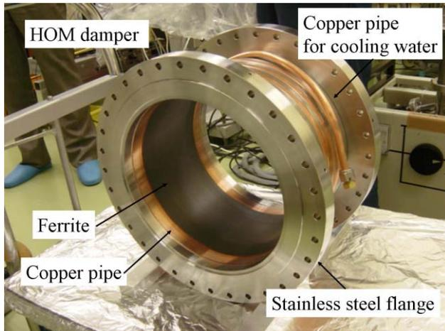
Figure 1: HOM damper for the crab cavity.
