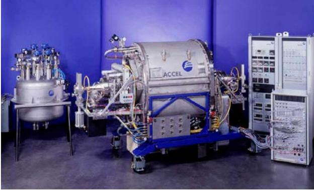
Figure 3: Cornell type module with valve box and LLRF
