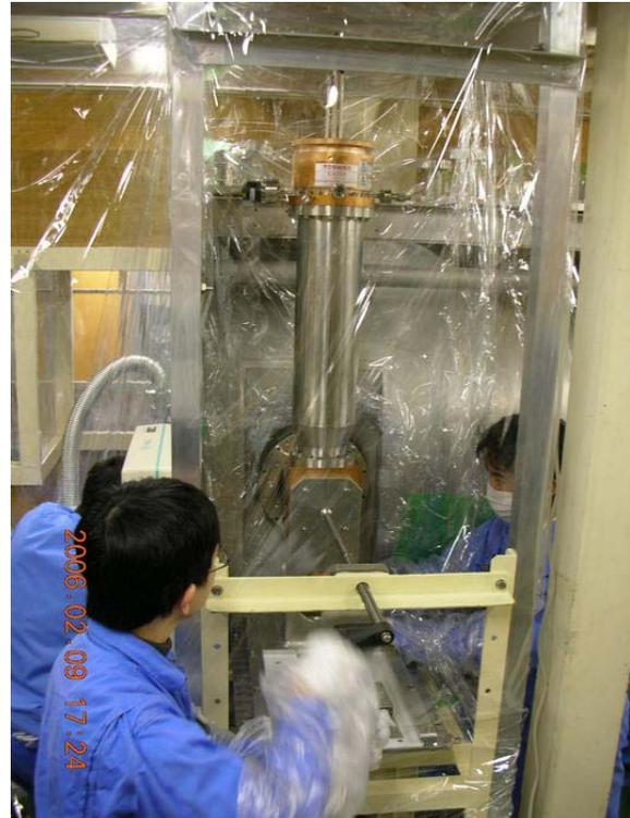
Figure 9: The input coupler is inserted into the cryostat.
