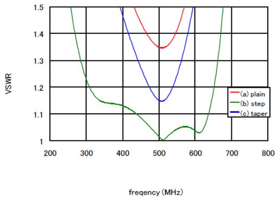
Figure 3: Transmit spectrum of T-stub structure.(a)The minimum value of the reflection is the highest in these models.(b)The reflection is the smallest. The bandwidth is very large.(c)The minimum value of the reflection and bandwidth are in middle of these models.
