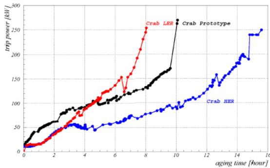
Figure 8: Progress of the traveling wave RF aging.
