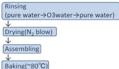
Figure 4: Prorcedure of The input coupler preparation.
