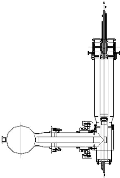
Figure 1: Schematic view of the RF input coupler
