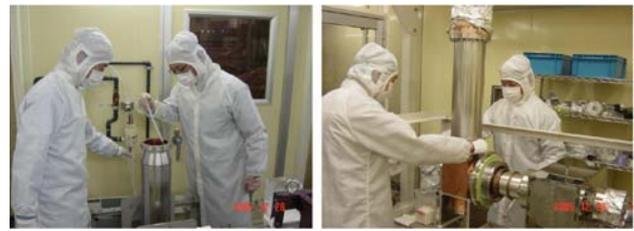
Figure 5: The input couplers are assembled in the clean room. (left) O<sub>3</sub> water rinsing. (right) The input coupler was attached to the aging stand.
