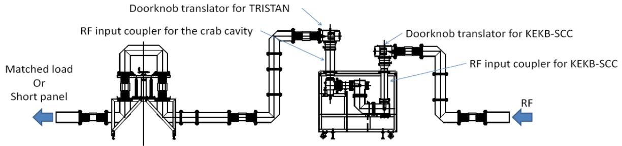
Figure 6: The Schematic view of the aging stand.
