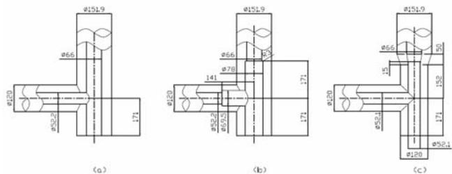
Figure 2: Schematic view of the candidates of the T-stub structures.(a)The simplest shape.(b)The diameters of inner conductor are changed at two points. (c)The diameter of inner conductor is changed using a taper.
