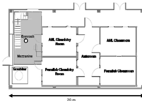
Figure 1: Layout of SCPF at ANL Bldg. 208
