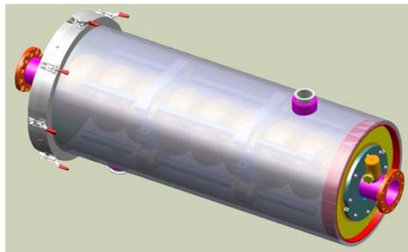
Figure 4: 1.3 GHz 9-cell cavity outside etching jacket.
