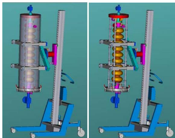
Figure 5: Transport cart holding cavity with and without etching jacket.
