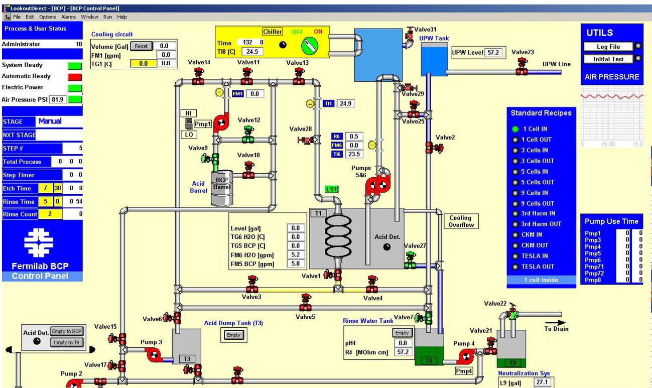
Figure 2: BCP System flow schematic. Operator GUI screen capture.
