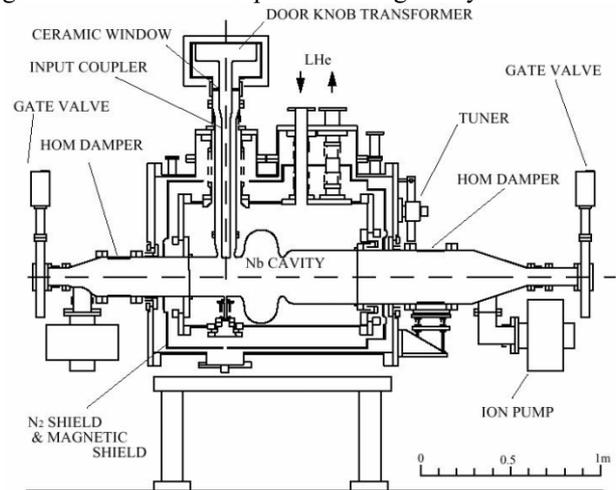
Figure 2: KEK-B Superconducting Cavity.
