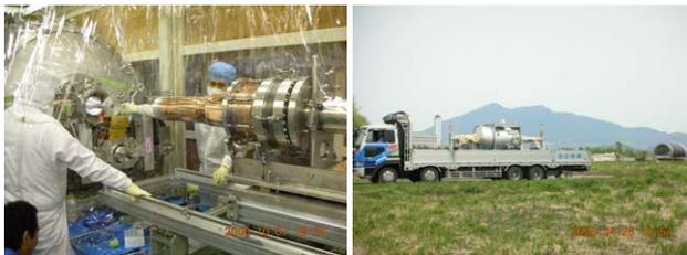
Figure 1: Photos of the assembly to the cryostat and the transfer to the horizontal test area.
