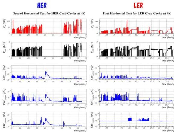
Figure 10: The time profile of the vacuum at the three cold cathode gauges (cavity/input coupler/coaxial beam pipe) during the RF processing.
