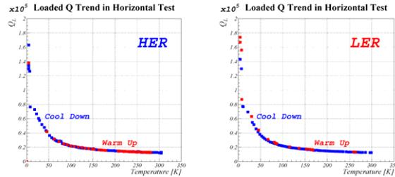
Figure 4: The loaded Q during cool-down and warm-up.
