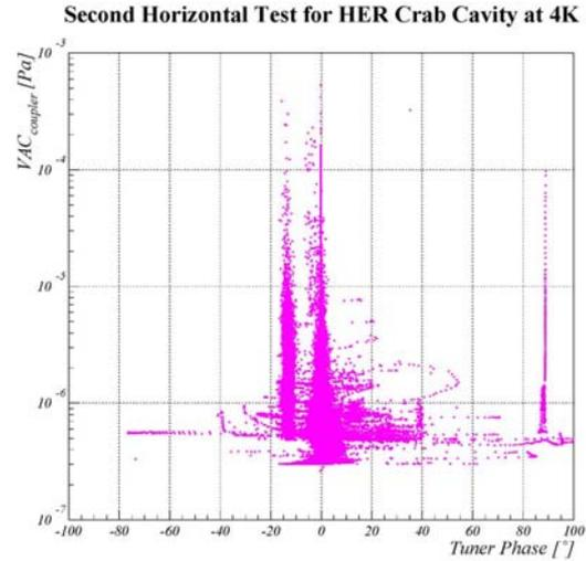
Figure 11: The correlation between the vacuum level and the tuner phase of the cavity during the conditioning.
