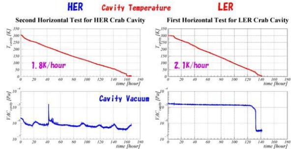
Figure 5: The time profile of the temperature and vacuum during cool-down.
