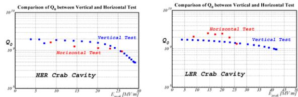
Figure 12: The comparison of  $Q_0$  vs.  $E_{peak}$  curve between the vertical and horizontal test.
