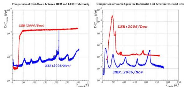
Figure 7: The vacuum vs. temperature during cool-down and warm-up.
