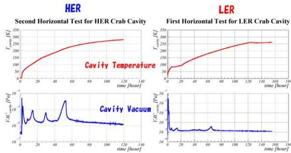
Figure 6: The time profile of the temperature and vacuum during warm-up.
