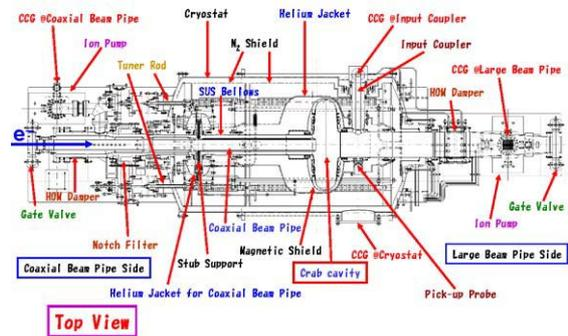
Figure 2: The assembly layout of Crab cavity.
