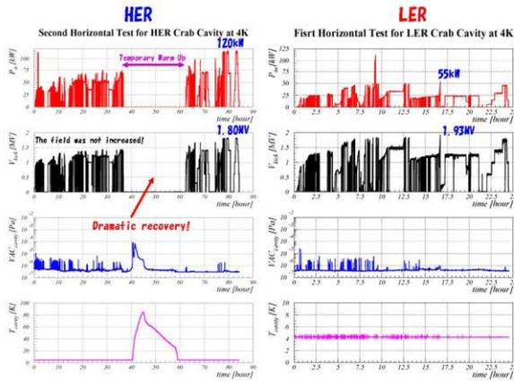
Figure 9: The time profile of the klystron power, the kick voltage, the vacuum and the temperature of the cavity during the RF processing.
