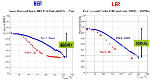
Figure 3: The frequency change during cool-down and warm-up.
