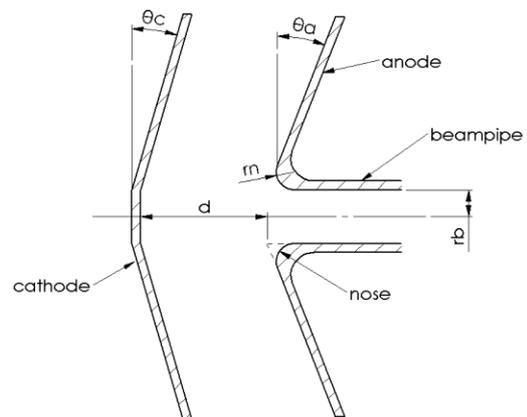
Figure 2: Schematic of the pierce structure.
