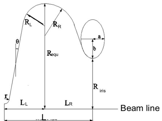
Figure 3: Shape of the first half cell of the sc cavity.
