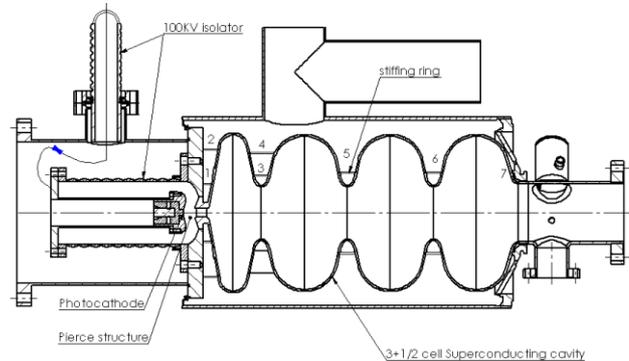
Figure 1: core elements of the upgraded photocathode injector.
