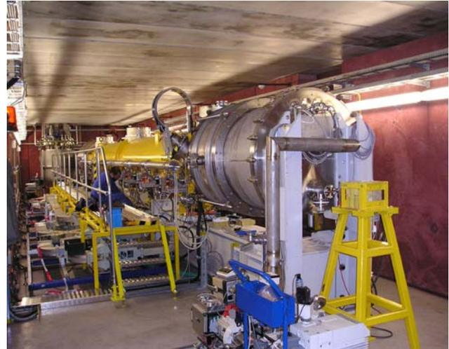
Figure 2: FLASH LINAC SRF module on the CMTB.
