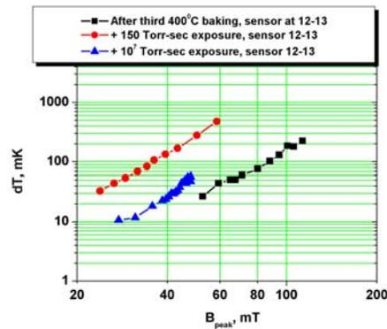
Figure 12: Thermometry data for the third set of experiments: after third 400°C baking, after the cavity was exposed to  $\approx 150$  Torr·sec, after the cavity was exposed to  $\approx 10^7$  Torr·sec
