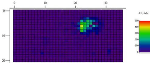
Figure 10: Temperature map at  $B_{peak}=115$  mT after the cavity was exposed to  $\approx 10^7$  Torr·sec.
