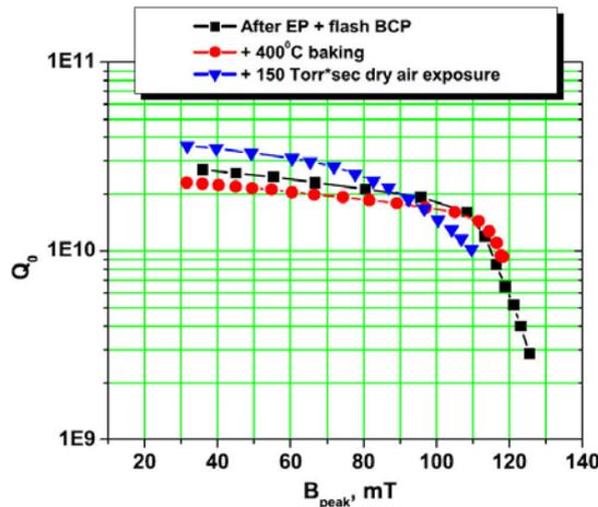
Figure 1: Quality factor versus peak magnetic field for the first three tests: after chemical treatment the excitation curve has a typical medium- and high-field Q-slope, after the cavity was baked at 400°C, after the cavity was exposed to  $\approx 150$  Torr·sec of dry air.
