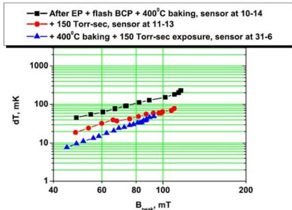
Figure 6: Thermometry data from the regions with high surface resistance after 400°C baking, that shows improvement of this regions by short exposure: after first 400°C baking, after first 150 Torr-sec air exposure, after second 150 Torr-sec air exposure.
