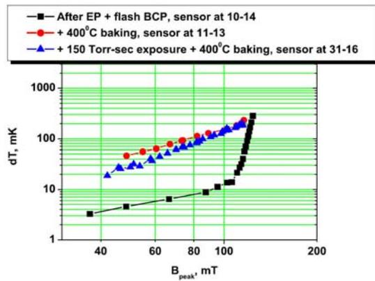
Figure 5: Thermometry data from the regions that showed high surface resistance: after chemistry, after first 400°C baking, after second 400°C baking.
