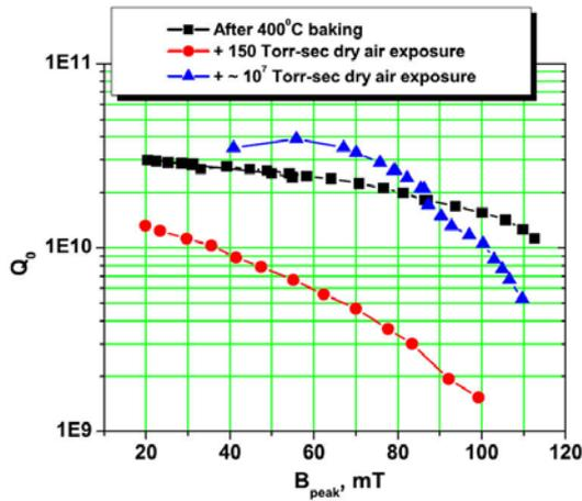
Figure 9: Quality factor versus peak magnetic field for the second group of three tests: after the cavity was baked at 400°C, after the cavity was exposed to  $\approx 150$  Torr·sec of dry air, after the cavity was exposed to  $\approx 10^7$  Torr·sec
