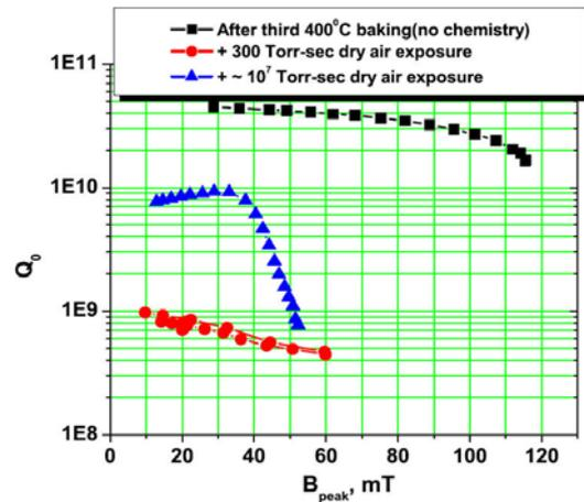
Figure 11: Quality factor versus peak magnetic field for the third group of three tests: after the cavity was baked at 400°C, after the cavity was exposed to  $\approx 300$  Torr·sec of dry air, after the cavity was exposed to  $\approx 10^7$  Torr·sec
