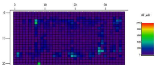
Figure 14: Temperature map at  $B_{peak}=48$  mT after  $\approx 10^7$  Torr-sec
