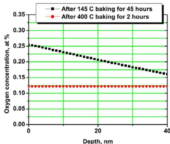
Figure 15: Diffusion calculation based on the modified oxygen pollution model proposed by G. Ciovati.
