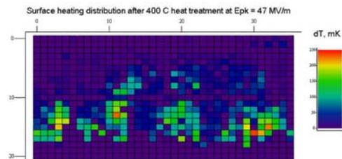
Figure 3: Temperature map at  $B_{peak}=117$  mT after the cavity was baked at 400°C.
