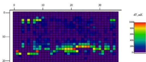
Figure 13: Temperature map at  $B_{peak}=50$  mT after the cavity was exposed to  $\approx 150$  Torr-sec
