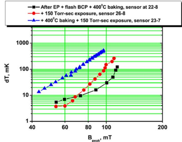
Figure 8: Thermometry data from the regions that showed anomalous losses after short exposures: after first 400°C baking, after the cavity was exposed to  $\approx 150$  Torr-sec, after the cavity was exposed to  $\approx 150$  Torr-sec following a second 400°C baking.
