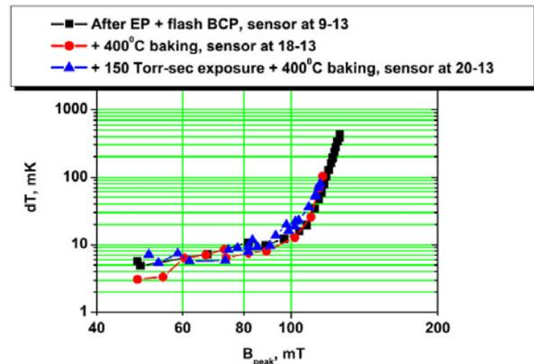
Figure 4: Thermometry data from the regions that showed high field Q-slope: after chemistry, after first 400°C baking, after second 400°C baking.
