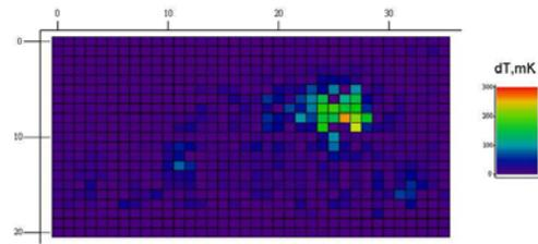
Figure 7: Temperature map at  $B_{peak}=110$  mT after the cavity was exposed to  $\approx 150$  Torr-sec.
