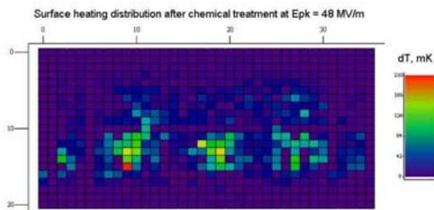
Figure 2: Temperature map at  $B_{peak}=117$  mT after the chemistry show three broad hot-spots.
