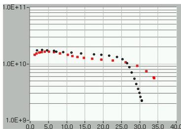
Figure 4: Q(E)-curves of 1DE5 before and after bake (some FE present before and after bake),GIREDMET
