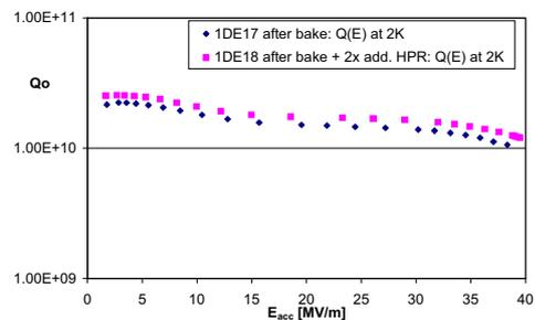
Figure 2:  $Q_0/E$ -curve of 1DE17 and 1DE18 at 2K after bake (and additional 2x HPR), NINGXIA
