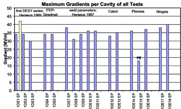
Figure 6: Maximum Gradients of all single-cell, fine grain Cavities
