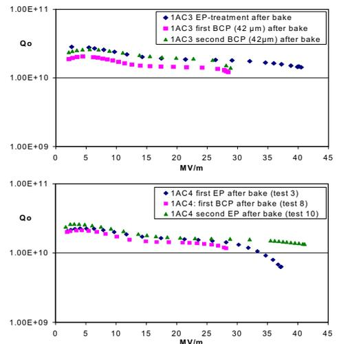
Figure 7: EP versus BCP by means of Q/E-measurement (1AC3 and 1AC4)
