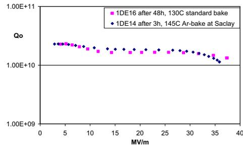
Figure 1:  $Q_0/E$ -curve of 1DE14 + 1DE16 at 2K after bake, PLANSEE
