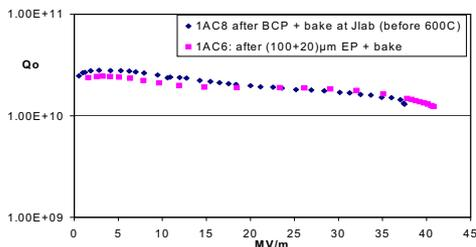
Figure 8: Q/E-curves of 1AC6 and 1AC8
