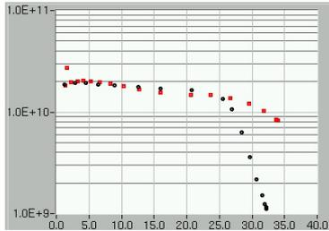
Figure 3: Q(E)-curves of 1DE4 before and after bake (some FE present before and after bake),GIREDMET
