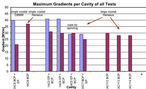
Figure 9: Maximum Gradients of all large grain and single crystal Cavities.
