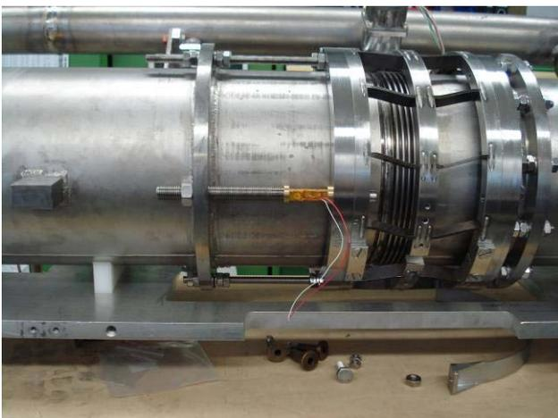
Fig. 9 - The Slim SS Blade tuner completely installed, piezo actuators are in place and preloaded.
