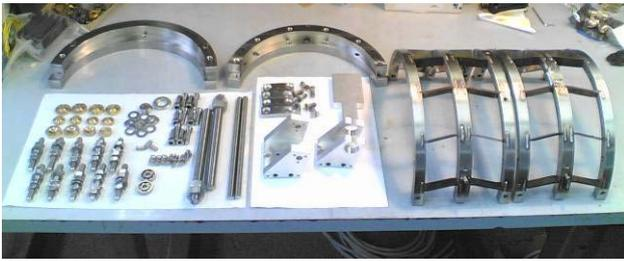
Fig. 7 – Tuner components before assembling
