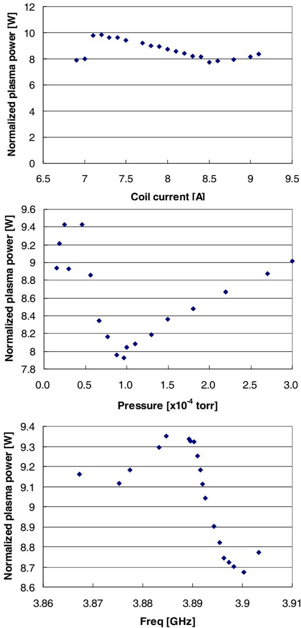
Figure 5. The normalized plasma power absorption at 10 W RF input power; top: Ar pressure  $1.0 \times 10^{-4}$  Torr; middle: Ar pressure  $1.0 \times 10^{-4}$  Torr and Coil current 8.5 A; bottom: Ar pressure  $4.4 \times 10^{-4}$  Torr and coil current 8.6 A
