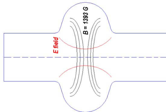
Figure 1: A simple illustration of a 3.9 GHz RF cavity with external dipole magnetic field of 1393 Gauss in the center to form the ECR condition.
