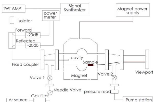
Figure 3: Schematics of plasma excitation in a cavity and sample placement.
