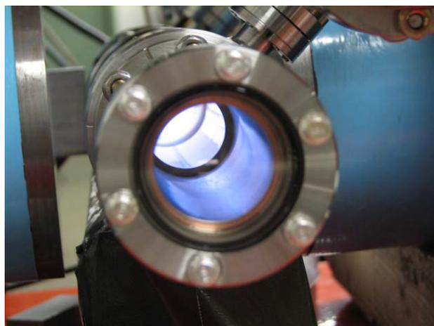
Figure 4. Light of Argon plasma through cavity view port
