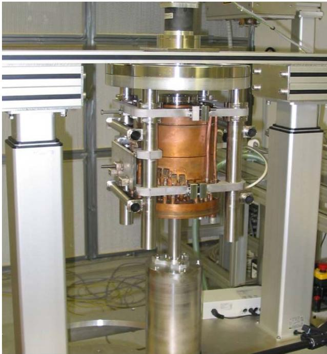
Figure 6: Vertical cleaning set-up for copper rf gun cavities
