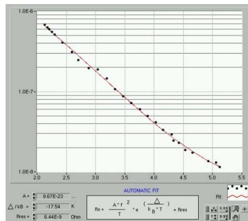
Figure 1: Q(T) curve of cavity 1AC9 after quick cooldown. Standard Q values and residual resistance were reached.
