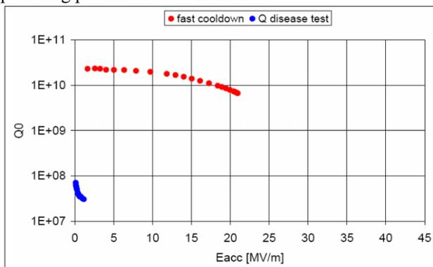
Figure 2: Test result of cavity 1AC9. After a fast cooldown (red dots) the cavity showed good performance and Q values above  $1 \cdot 10^{10}$  for accelerating gradients below 18 MV/m. At 22 MV/m the cavity was limited by quench. For a second test the cavity was cooled down very slowly resulting in very low Q values and gradients, indicating that the niobium of the cavity was contaminated with hydrogen (Q disease).
