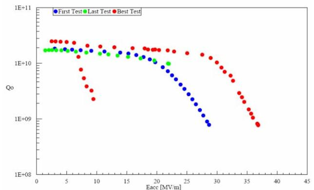
Figure 4: RF test results of cavity 1AC1. First test (blue dots), achieved with standard BCP treatment, Best test (red dots) achieved with standard electro polishing treatment and last test (green dots) achieved with new electro polishing method. During the last test, at 22 MV/m a quench limited the cavity to reach higher fields. Multipacting was observed from 19 MV/m on during that test.
