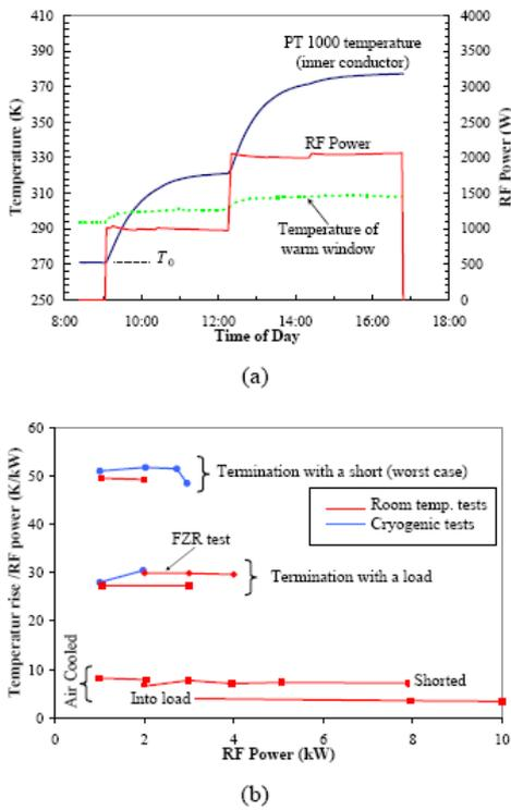
Figure 7: CW measurements at the TTF-III type coupler. (a) Example of PT1000's temperature versus time. Measurements were made with HoBiCaT cold and the waveguide shortened. (b) Summary of all tests.
