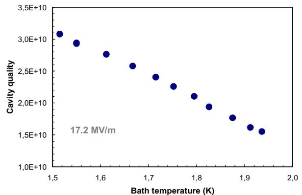
Figure 6: Unloaded quality factor of the TESLA cavity versus bath temperature. At low temperatures the quality factor increases. There is no saturation by other loss mechanisms seen at these measurements at HoBiCaT.
