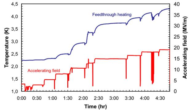
Figure 9: Temperature rise of the sapphire HOM feedthroughs and accelerating field versus time of the S33 cavity in CW operation. The HOM heating is at a moderate level.
