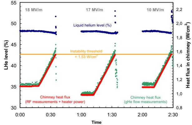
Figure 3: By using a electrical heater the total losses (red) of the heater and the dissipated cavity wall losses for different field settings (blue) were increased. The quenching occurred at total power of 35 W or 1.53 W/cm<sup>2</sup> in the chimney.
