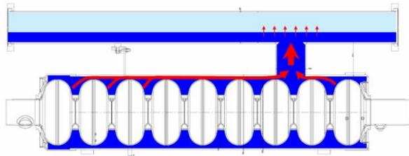
Figure 2: Layout of the helium vessel.
