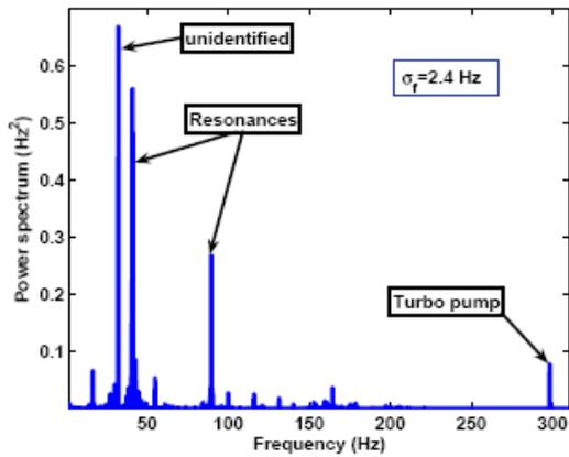
Figure 10: Power spectrum of microphonics
