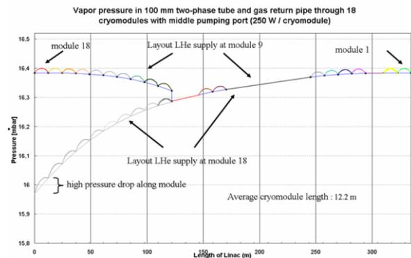
Figure 4: Pressure drop along the gas return pipe calculated for the BESSY FEL. Feeding the helium at the end of the linac will cause high pressure drop along the modules at the end. Supplying the helium in the middle of the linac gives better results.
