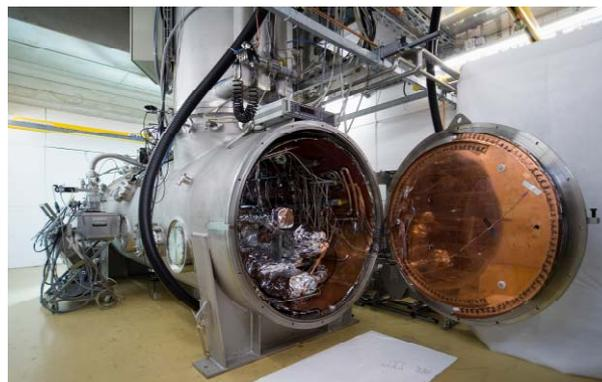
Figure 1: The cryostat of the HoBiCaT facility for CW operated SC TESLA cavities
