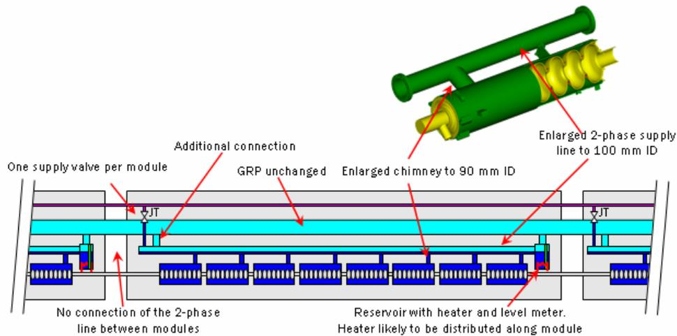
Figure 5: Design of a CW cryo module
