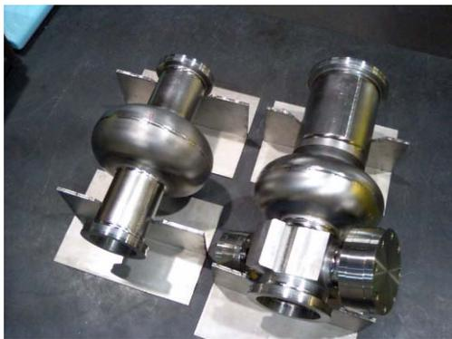
Figure 7: Nb test cavities of C-single and E-single.
