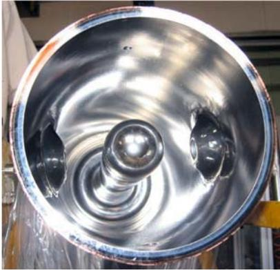
Figure 5: The new cavity after being Nb sputtered
