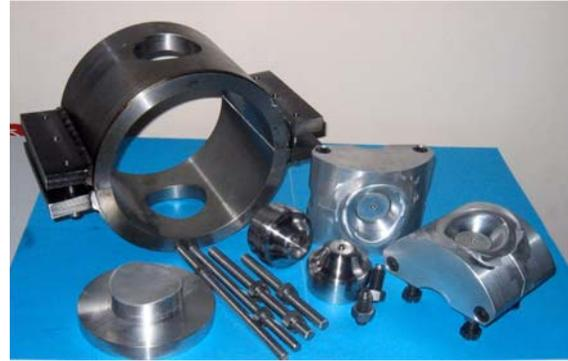
Figure 3: Cage, dies and punches used for deforming the beam port area of the new medium  $\beta$  cavity
