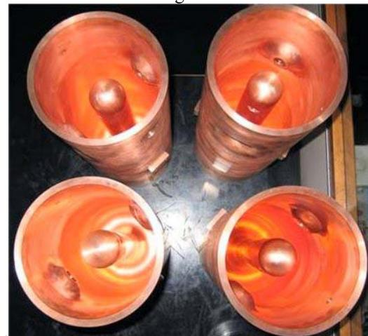
Figure 4: The four cavities after the beam port shaping
