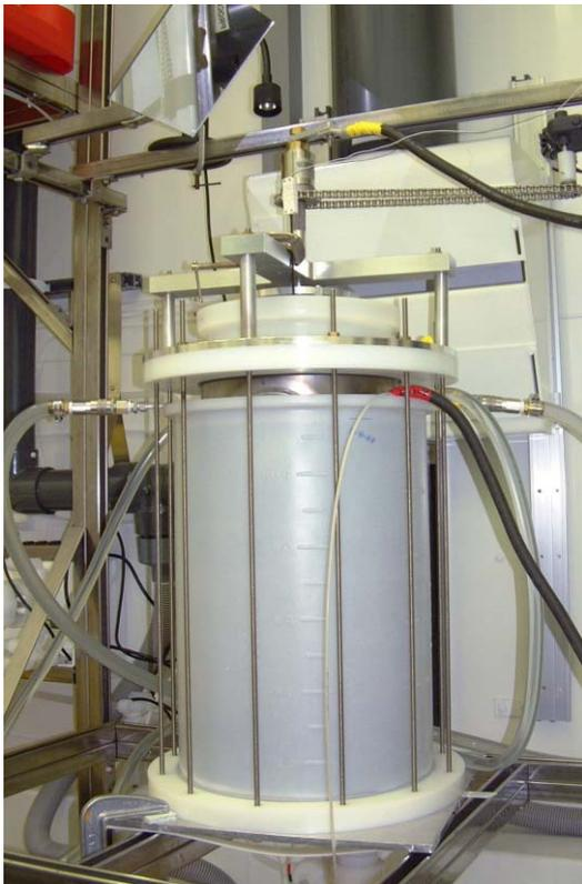
Figure 4: QWR EP system ready for procedure.
