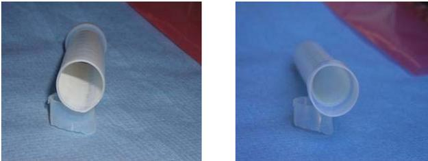
Figure 7: Sulphur removal with ethanol. Left: tube as removed from EP apparatus; right: tube after ethanol cleaning
