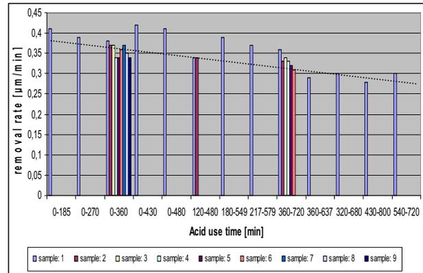
Figure 5: Reduction of removal rates correlated to the in use time of the acid
