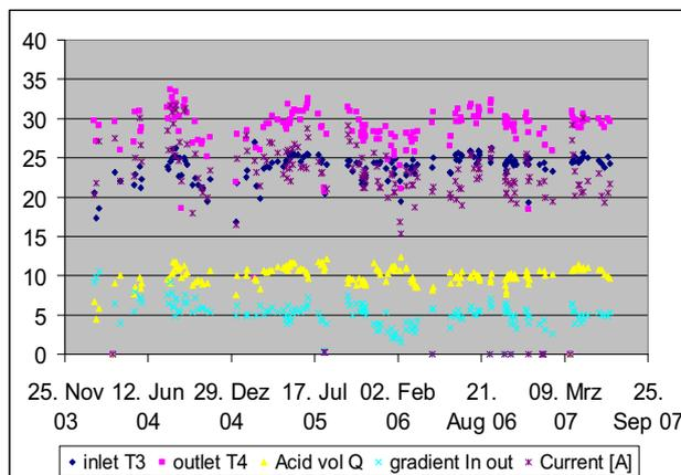
Figure 3: Correlation of average current, acid temperature and temperature gradient since 2003
