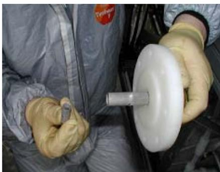
Figure 3: Impeller section detached form sensor due to corroded connectors
