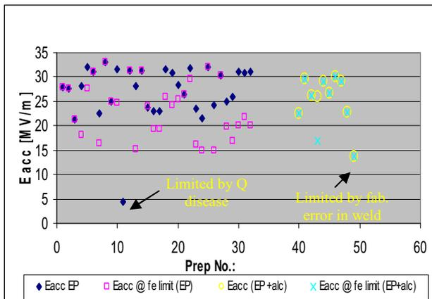
Figure 8: Comparison of test results with and without alcohol rinse applied after assembly before 6 times HPR (only RF test results 1st power rise before 120 C baking are displayed)
