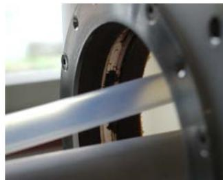
Figure 1: Corrosion of rotary shaft seals made from Viton the PVDF material.
