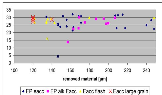
Figure 6: Correlation of max. gradient and removed material since 2004. (only RF test results 1st power rise before 120 C baking are displayed)
