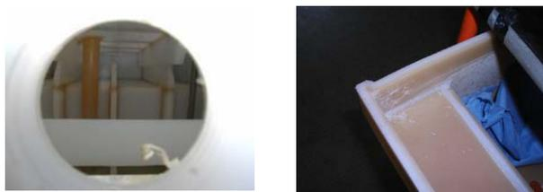
Figure 2: Left corrosion on welds of sump no 2; Right corrosion on the commercial available PVDF
