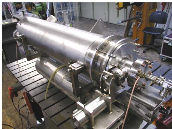
Figure 5: cavity and vessel installed in alignment fixture, (tank brackets and power coupler port settling on fixture)
