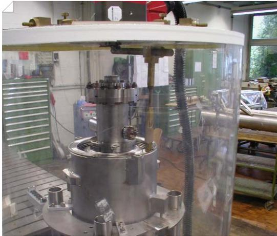
Figure 6: Cavity installed in Argon cabin with orbital arm and tungsten electrode
