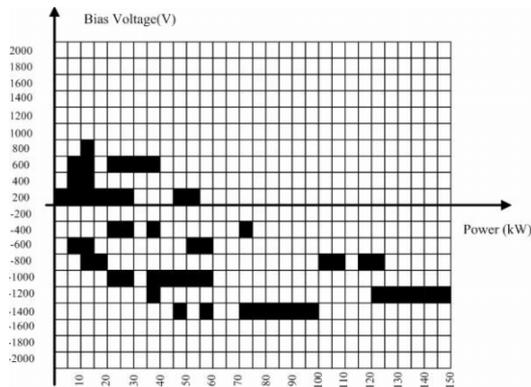
Fig.8: The vacuum variation during the DC bias voltage conditioning, the filled blanks indicate vacuum pressure increasing
