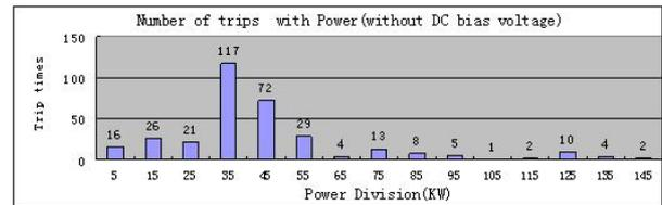
Fig.5: The trips times as a function of power
