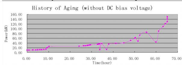
Fig.4: The history of conditioning without DC bias voltage
