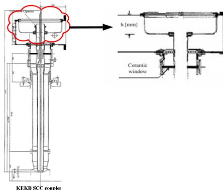
Fig.1 High power input coupler for BEPCII SCC is based on the KEKB SCC coupler [2].
