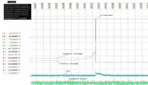
Fig.7: Inspection screen during the DC bias voltage conditioning
