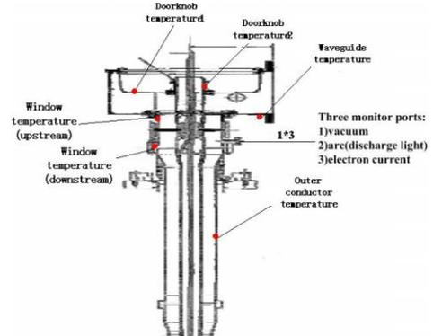
Fig.3 The distribution of various monitor sensors
