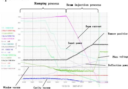
Fig9: Inspection result of DC bias voltage processing with beam operation
