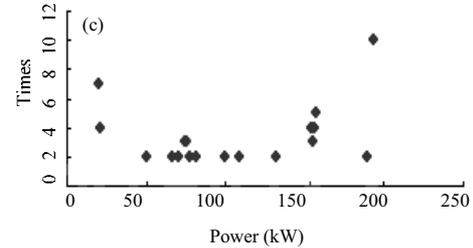
Fig.2 Trip times as a function of the power level during the initial test
