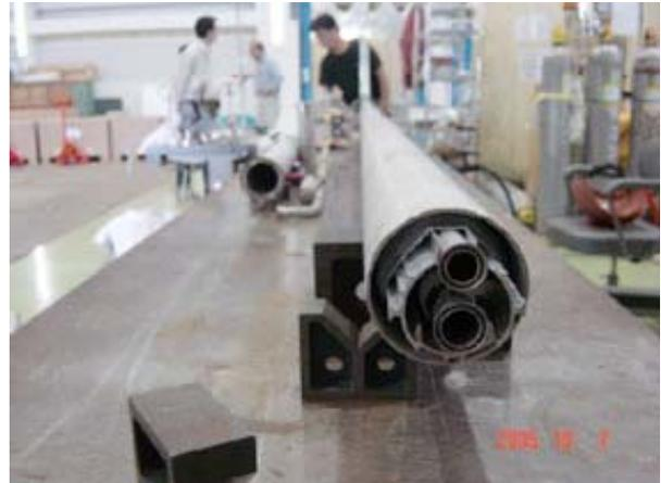
Figure 9: A photo of a transfer line under manufacture.
