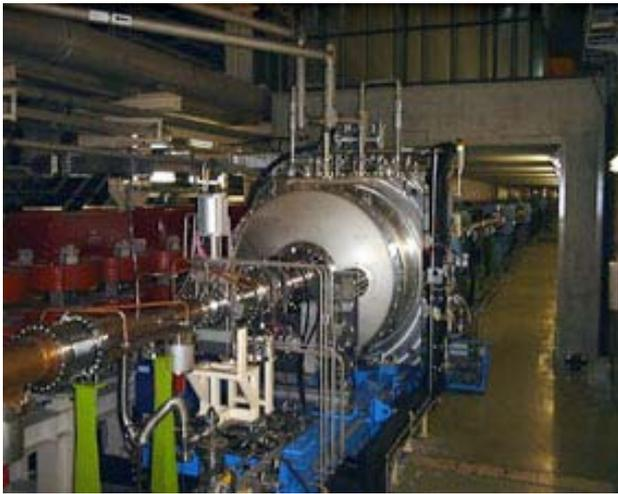
Figure 5: Crab cavity cryostat in HER.
