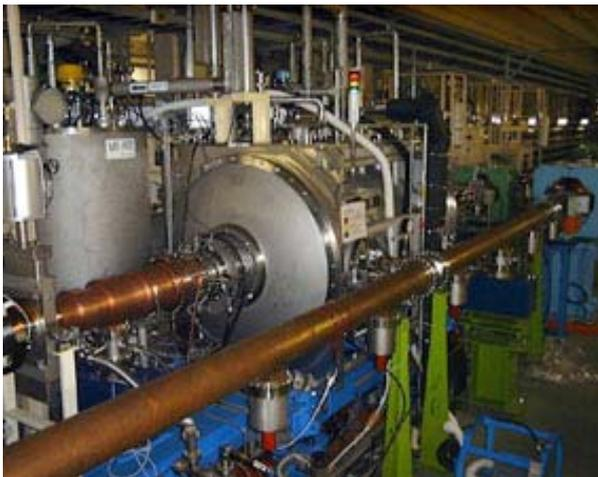
Figure 7: Crab cavity cryostat in LER.
