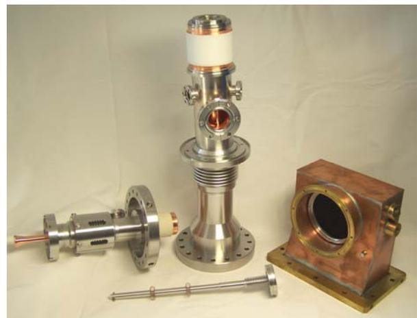
Figure 2: Coupler parts and sub-assemblies: cold coax, warm coax, tuning pushrod and waveguide box (from left to right).
