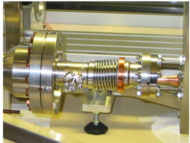
Figure 5: Coupler cold bellows lateral deformation.
