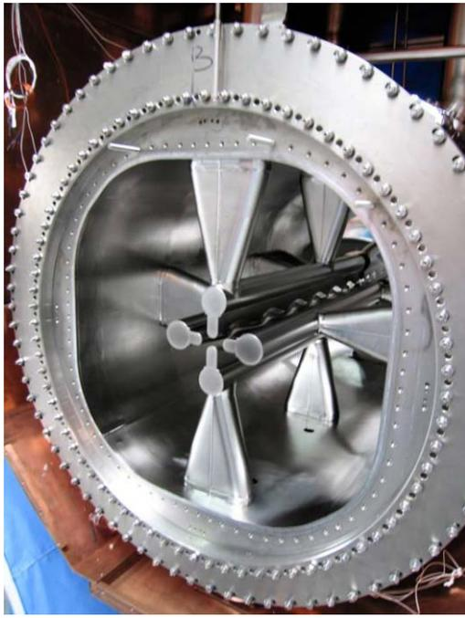
Fig.5: photo of one SRFQ in the on-line cryostat; the resonator is surrounded by its own liquid He dewar; the Cu thermal shield at 77 K can be seen
