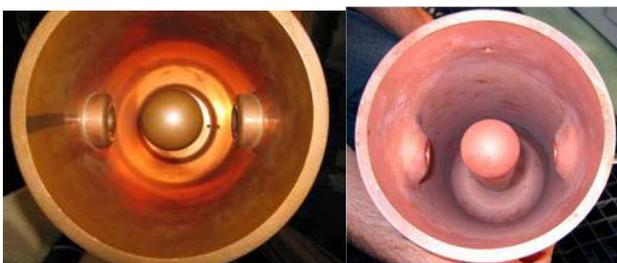
Fig.3: the figure shows the improvements, introduced in the upgraded prototype Cu-base of medium  $\beta_0$  resonators, so as to improve the quality of the Nb layer and hence the Q-vs- $E_a$  curve.
