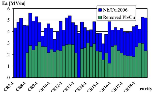
Fig.2: distribution of medium  $\beta_0$   $E_a$  values before (green bars) and after (blue bars) replacement of Pb with Nb as SC layer. The average value increased by more than 60%.
