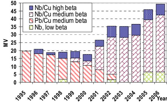
Fig.9: variation of ALPI equivalent voltage in the last 12 years; the relative contributions of the three  $\beta_0$  sections is highlighted (replacement of Pb with Nb in medium  $\beta_0$  resonators being the most relevant one)
