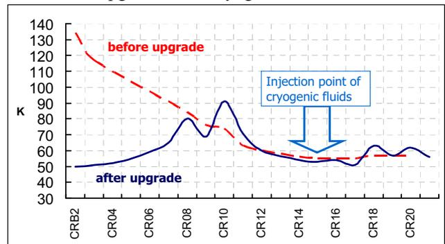
Fig.7: distribution of the gas He shield temperatures of ALPI cryostats, with respect to the injection point, before and after the cryogenic lines upgrade
