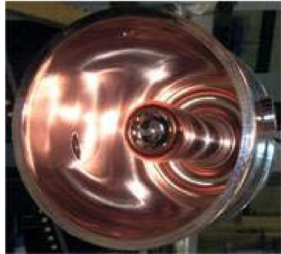
Fig.1: Cu base for Nb sputtered higher  $\beta_0$  resonators; the geometry is designed to be best suited to the deposition of a uniform Nb layer.
