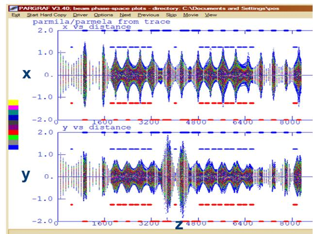
Fig.10: example of a PARMELA multiparticle simulation (transverse phase space envelope), calculated for a  $^{70}\text{Zn}^{10+}$  beam to be accelerated with Tandem-ALPI
