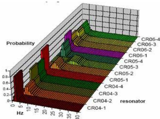
Fig.8: for each lower  $\beta_0$  QWR, the deviation probability of the actual resonant frequency with respect to 80 MHz was recorded and plotted
