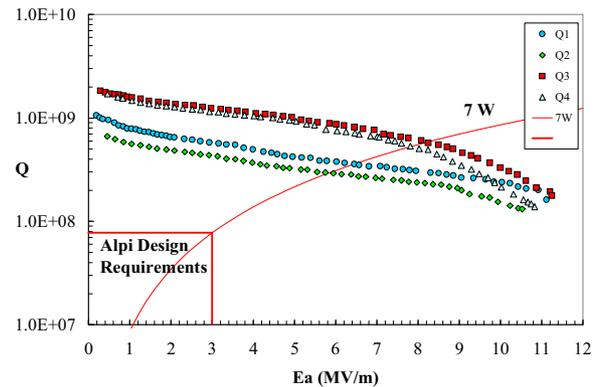
Fig.4: Q-curves of 4 out of the 12 80 MHz full Nb resonators, which were installed in ALPI in 1998.
