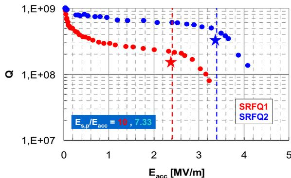
Fig.6: Q vs  $E_a$  curves of superconducting RFQs (SRFQ1 and SRFQ2); the figures shows the specified working point (at  $P_{diss} = 10$  W) (red and blue star), as well as the  $E_{s,p}/E_a$  ratios.
