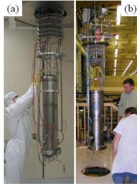
Figure 12: Photographs of (a)  $\beta_{opt} = 0.041$  and (b)  $\beta_{opt} = 0.085$  cavities on the RF test stand.
