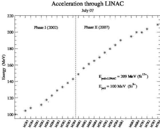
Figure 8. Energy gain by the Si beam from the Pelletron accelerator.
