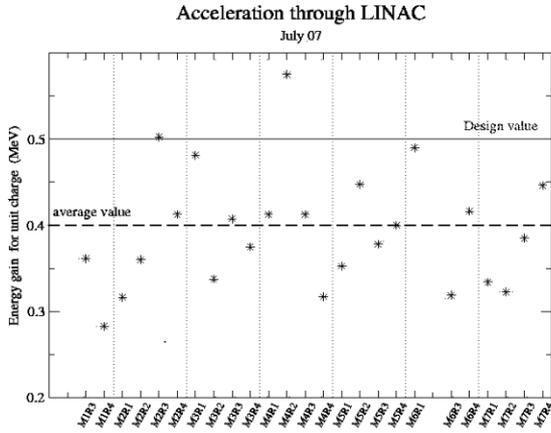
Figure 7. Energy gain through each QWR resonator for a Si13+ beam injected from the Pelletron.
