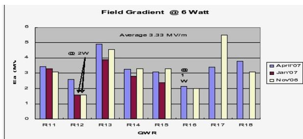
Figure 5. Field gradient achieved by 8 resonators on 3 on-line tests.
