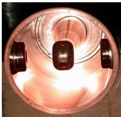
Figure 6. End view of the lead plated Cu QWR for BARC-TIFR Linac booster.
