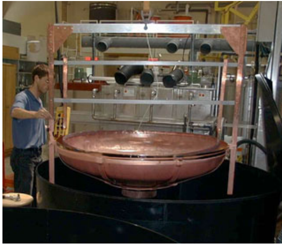
Figure 8: 200 MHz half-cell under preparation for electropolishing at CERN.
