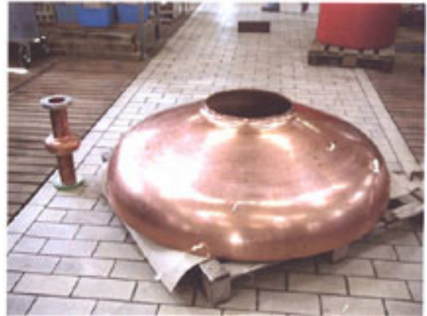
Figure 7: A comparison of the 200 MHz and 1500 MHz cavity sizes.
