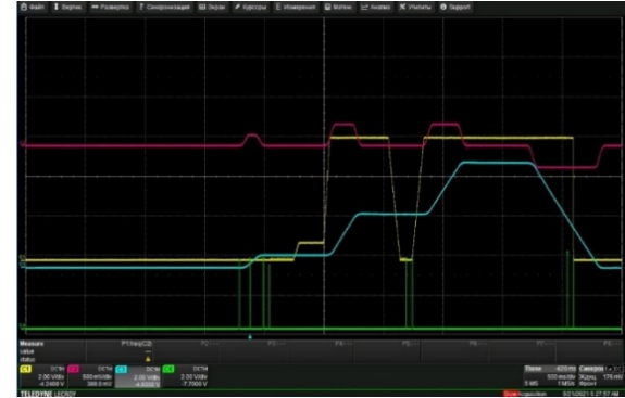
Figure 9: RF voltage applied to the falling magnetic field.
