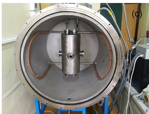
Figure 2: Niobium cavity inside of testing cryostat.
