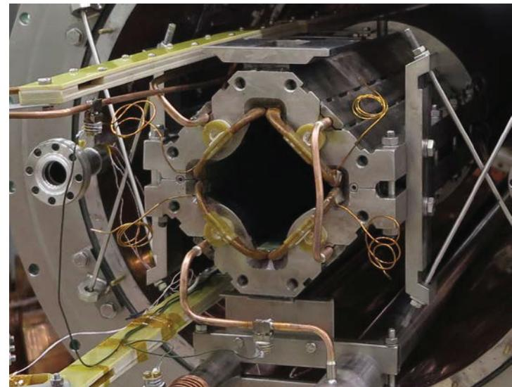
The Nuclotron-type design based on a cold, window-frame iron yoke and a winding of the hollow superconductor was chosen for the NICA Collider.
