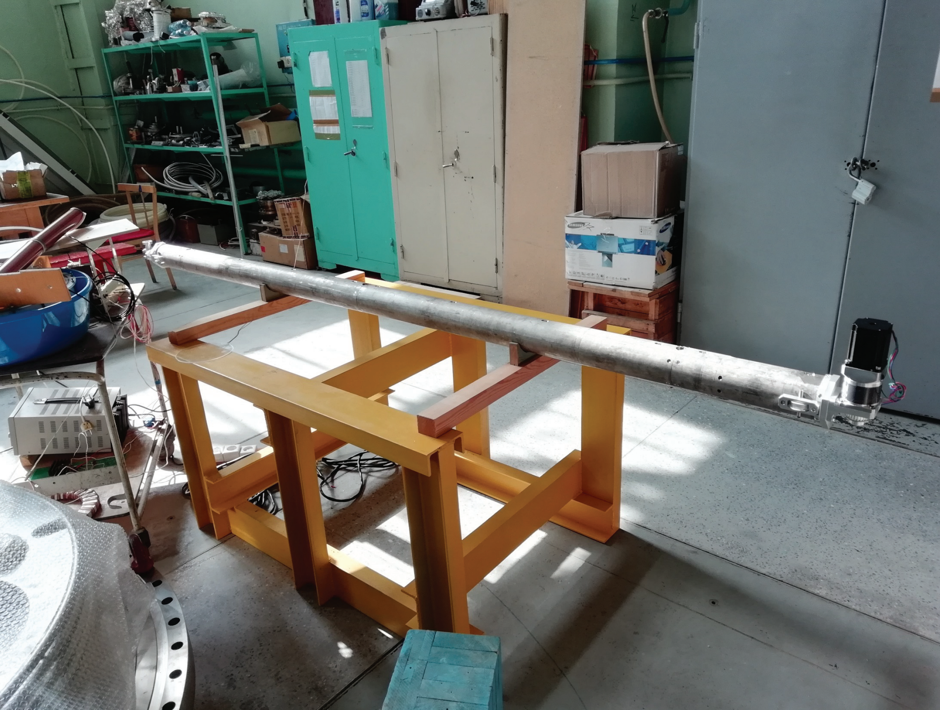
The mirror compass for measuring of the straightness magnet field line at cooling section
