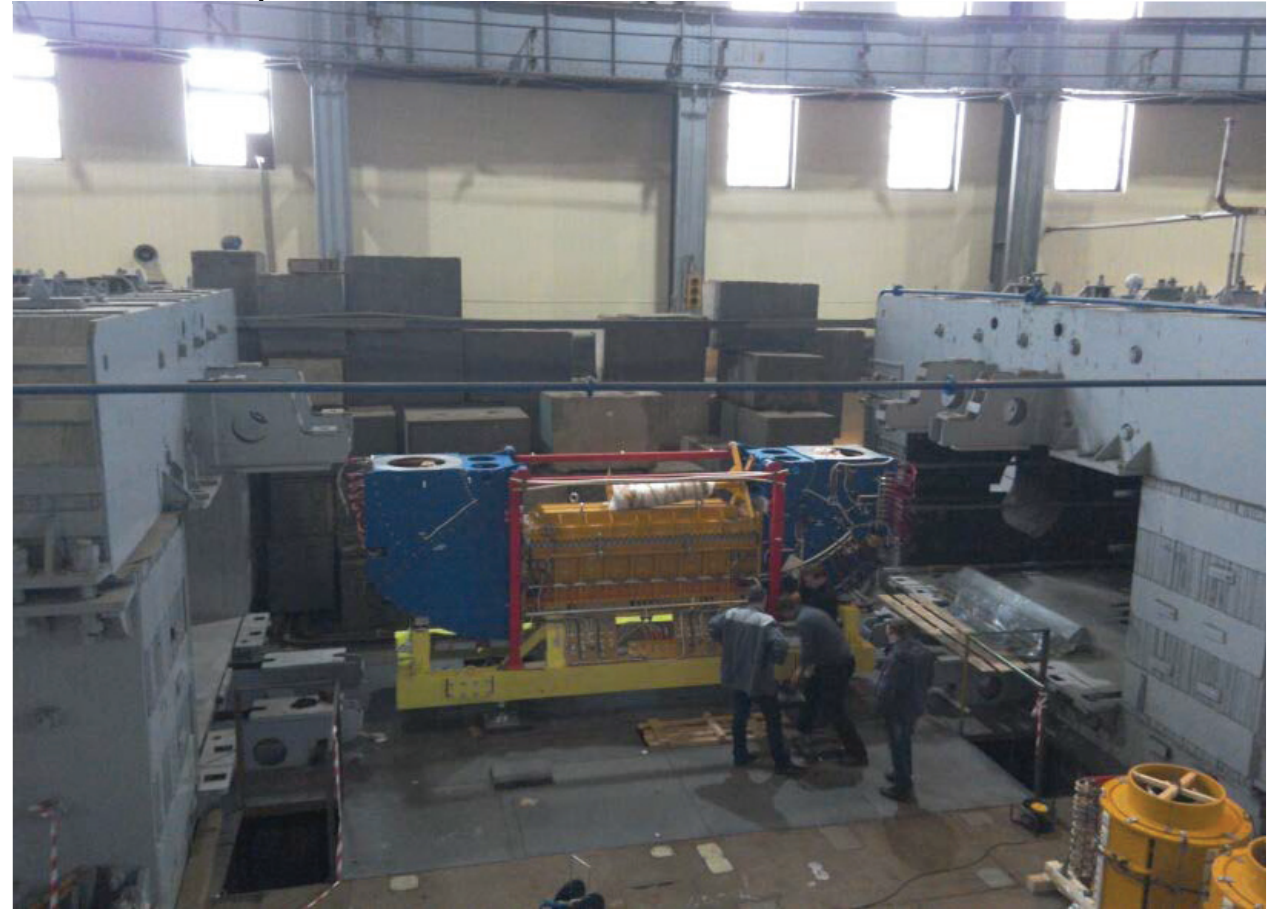
The cooler at nominal position at straight section NICA booster (gap between dipole magnet of synhrophasatron)
