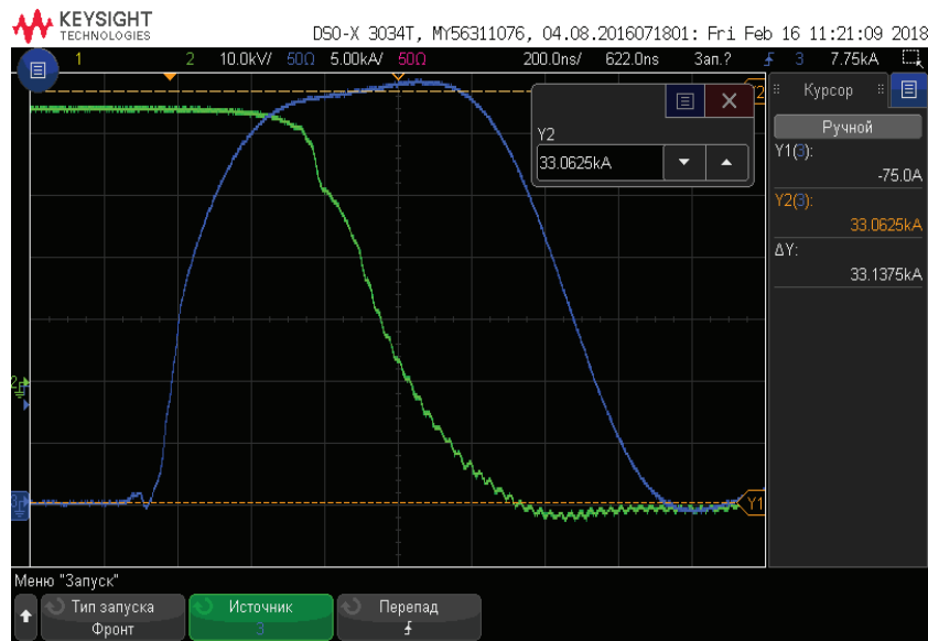
Oscillograms of current and voltage pulses during testing (200 ns/div)
