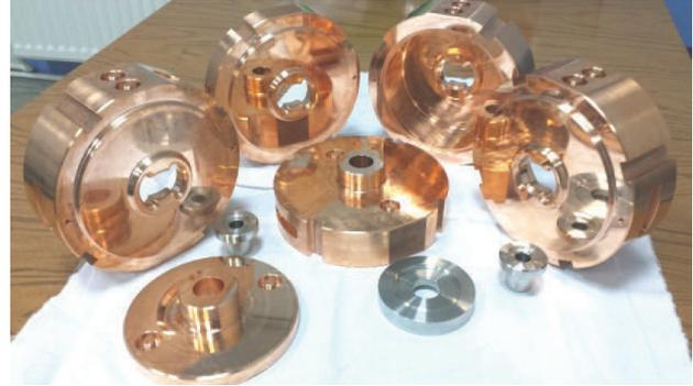
Figure 4: Parts of the cavity after machining.
