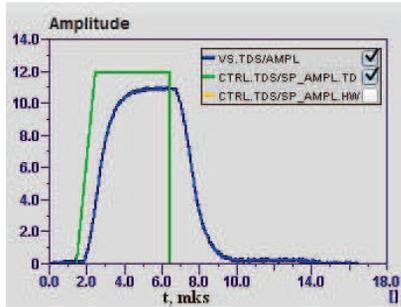
Figure 6: Envelopes of RF signals from the amplifier (green curve) and from the RF probe in the cavity (blue curve).
