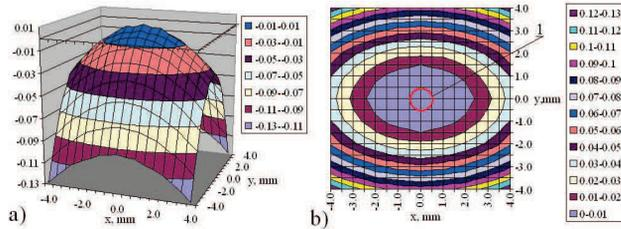
Figure 3: The surface of normalized deflecting voltage  $\frac{V_{d, 90^\circ}(x,y)}{V_{d, 0^\circ}(0,0)} \cdot 100\%$  (a) and corresponding contour map near the cavity axis (b), 1 - rms beam size of REGAE.
