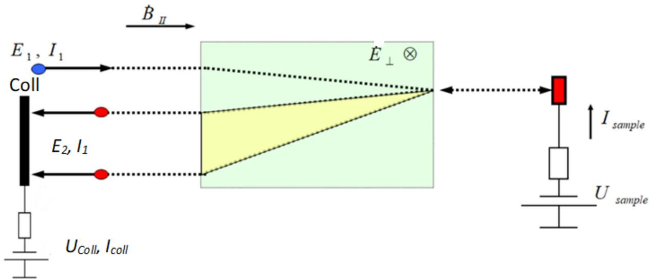
Figure 1: Principle scheme of measurement of  $K_{SEE}$ :  $E_1$  and  $I_1$  are the energy and current of the initial electrons,  $E_2$  and  $I_2$  are the energy and current of the secondary electrons which come to collector,  $U_{sample}$  is the potential of the sample,  $I_{sample}$  is the current of the source supplying the sample,  $E_{\perp}$  is the transverse electric field, and  $B_{\parallel}$  is the longitudinal magnetic field.
