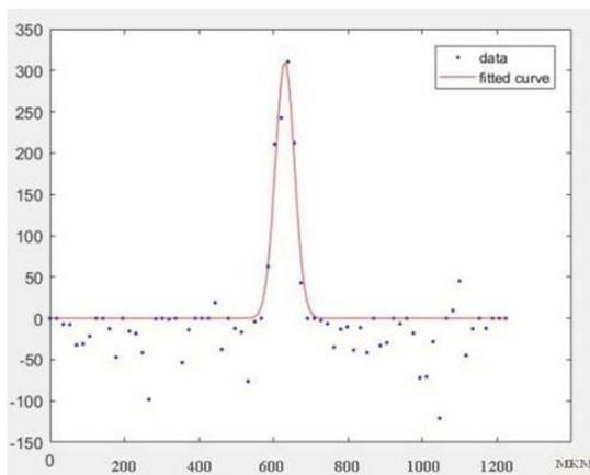
Figure 7: Measured blur function in the horizontal plane.
