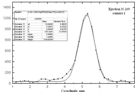
Figure 4: Measured blur function of the boundary for object with a thickness of 350  $\text{g/cm}^2$ .
