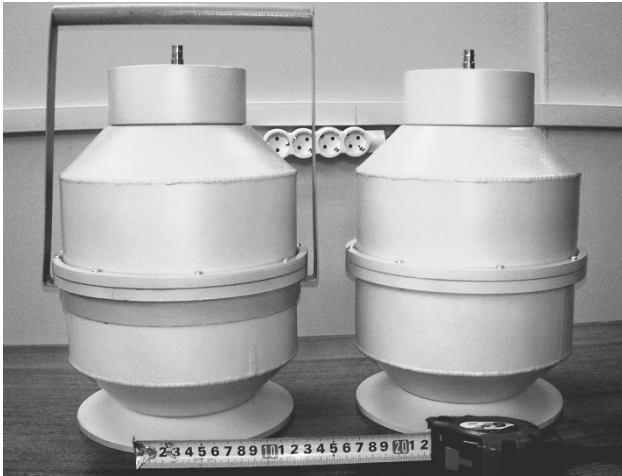
Figure 6: The first prototypes of the main and complementary detectors. Both have the same outer layout. The main detector on the photo is supplied with the removable handle.
