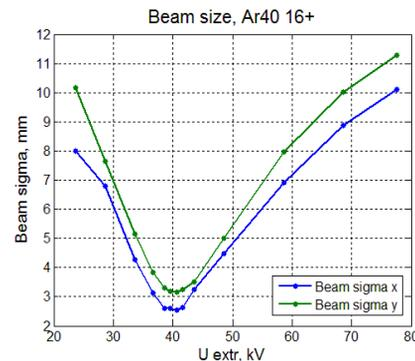
Figure 4: Beam size from accelerated voltages relations.
