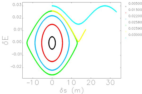
Figure 4: Phase trajectories for synchrotron oscillations.
