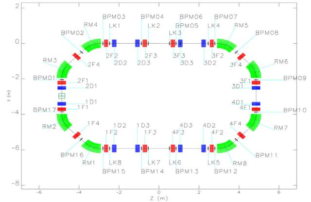
Figure 2: Damping Ring layout.
