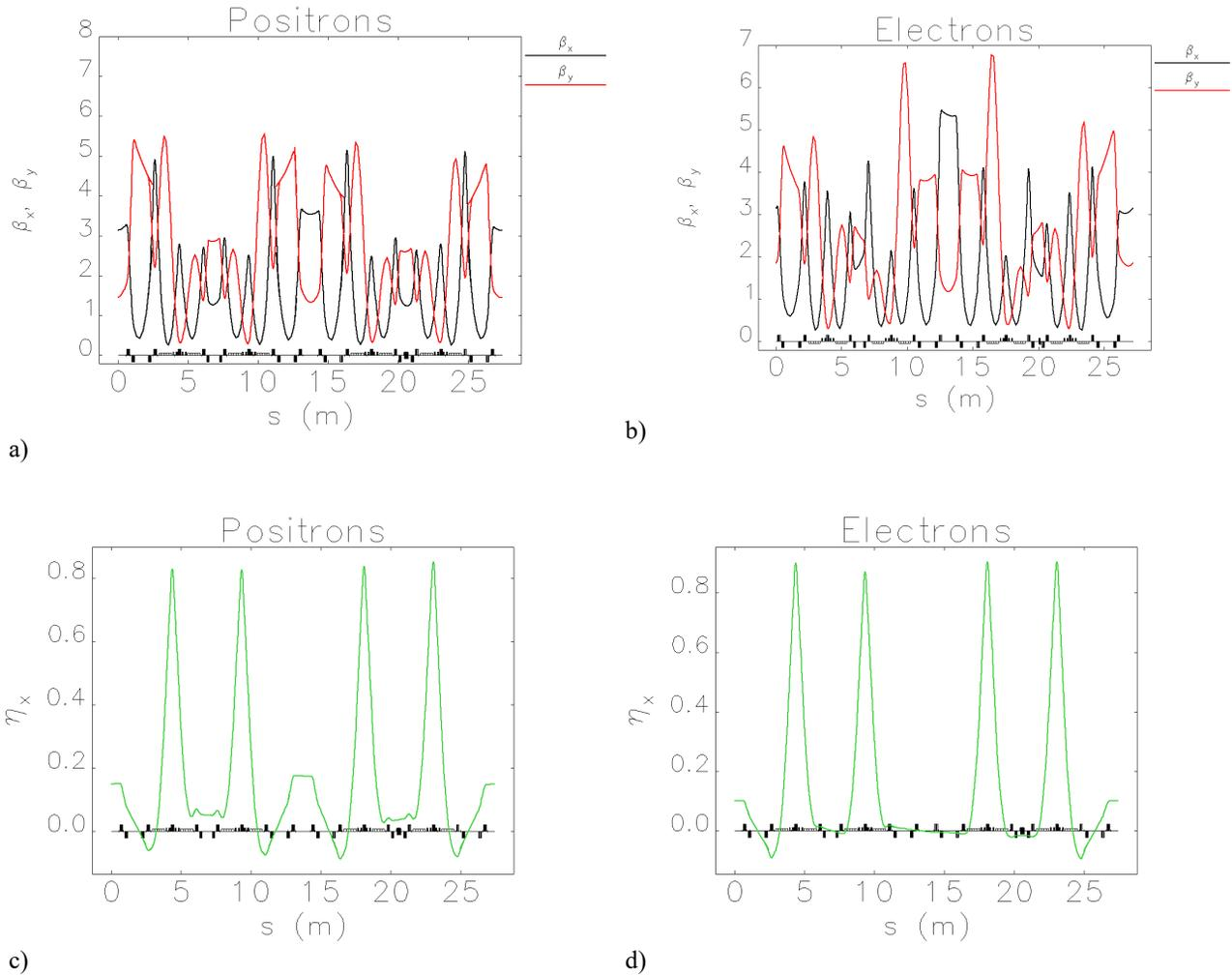
Figure 3: Optical and dispersion functions for Damping ring operation modes: a) positron beta-functions, b) electron beta-functions, c) dispersion of positrons, d) dispersion of electrons.
