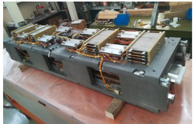
Figure 3: The overall view of 22-pole 7 T magnet of DELTA wiggler with quench protecting system.
