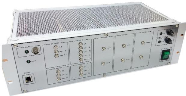
Figure 2: CPU module of LLRF controller.
