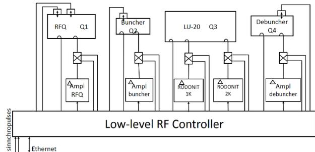
Figure 1: Injector of Nuclotron RF system.
