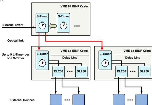
Figure 1: Synchronization structure using S-Timer and L-Timer modules.
