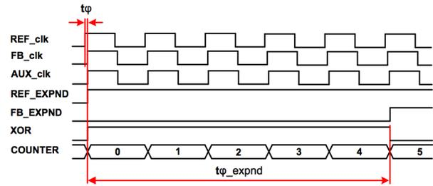
Figure 10: Time diagram of the stroboscopic phase measurement.
