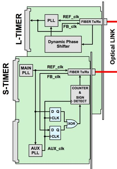
Figure 9: Block diagram of sub-nanosecond phase compensation.
