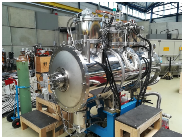
Figure 2: Superconducting 7 Tesla wiggler during site acceptance test in DELTA SR Source.
