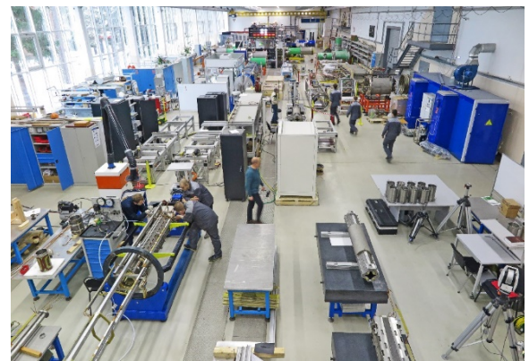
Figure 4: Line for assembling and cryogenic testing of SC-magnets.
