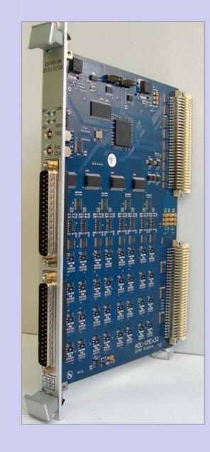
ADCx32 provides measurements of such parameters as HV charger voltage, PFN voltage, demagnetizer current and magnetic lens current of LIA-20 Pulsed HV System with 1540 total number of channels and 500us – 20ms time range.
