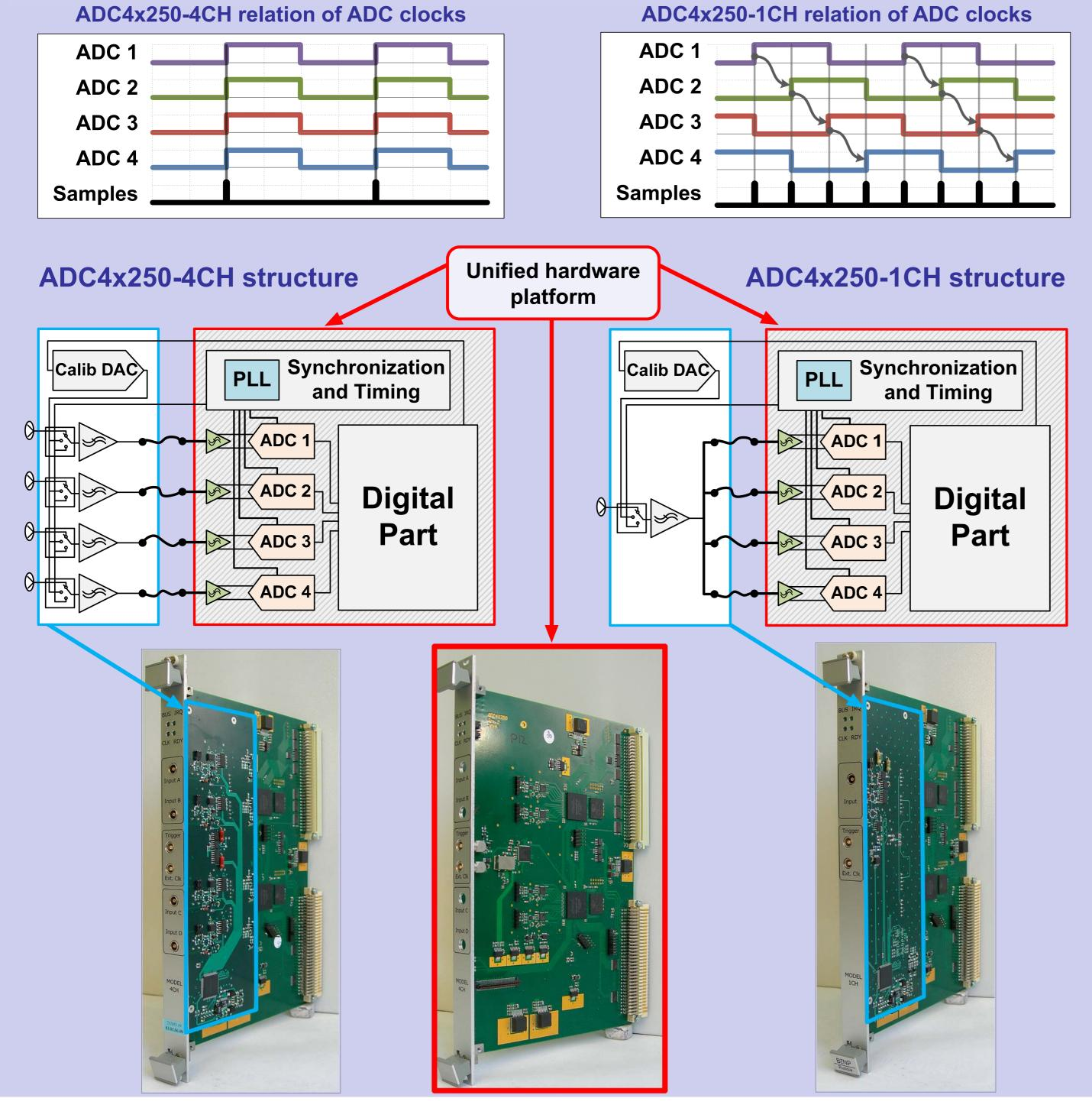
ADC4x250 is set of two devices. The first of them is four-channel 250 MSPS digitizer ADC4x250-4CH. Its structure is shown on the left side of illustrate. And the second one is one-channel device with performance of 1000 MSPS shown on the right and named ADC4x250-1CH.
