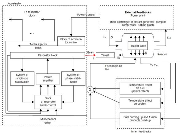
Figure 4: ADS structural scheme with feedbacks.
