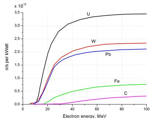
Figure 2: Neutrons/s per beam kWatt in photonuclear and photo fission reactions from Bremsstrahlung photons for an electron beam.
