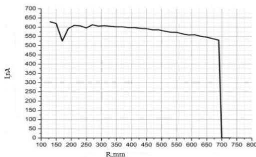
Figure 2: Radial dependence of the accelerated ion beam
